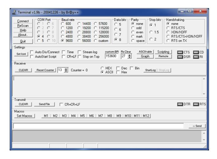
Terminal should find available COM Ports automatically. If the port number buttons are all gray, confirm that another program isn't using the desired port and click the ReScan button. As shown above, select an available COM Port, set Baud Rate to 9600, Data bits to 8, Parity to none, Stop bits to 1, and Handshaking to none. Click **Connect** – the same button should now say **Disconnect**. The **CTS** indicator turns green at this time, but it's safely ignored.
